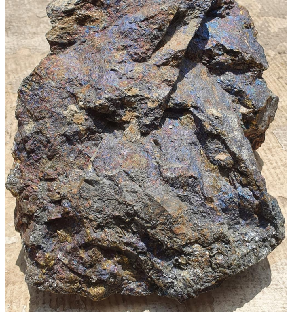
Sampled rock from previously mined polymetallic deposit showing massive sulphides including bornite, malachite and chalcopyrite
