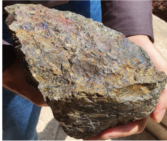
Sampled rock from previously mined polymetallic deposit showing massive sulphides including bornite, malachite and chalcopyrite
