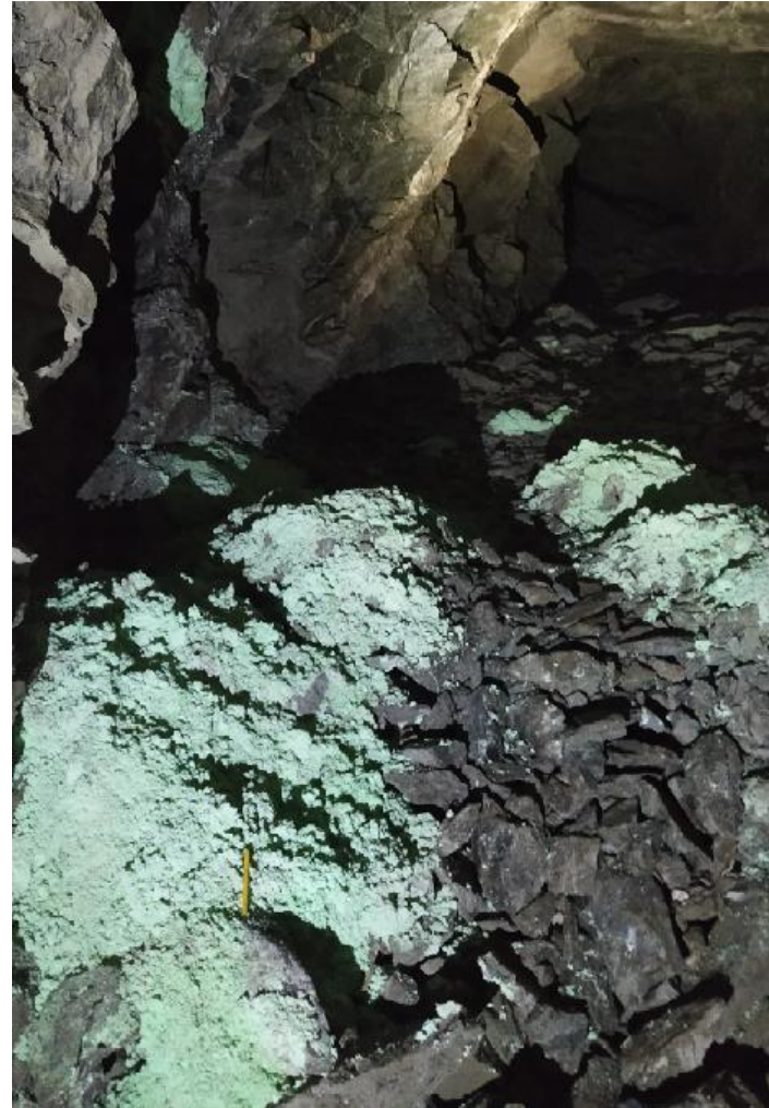
Below: Powdery, greenish nickel oxide minerals on the gallery wall and rocks on the gallery floor. Yellow magnetic pen for scale.
