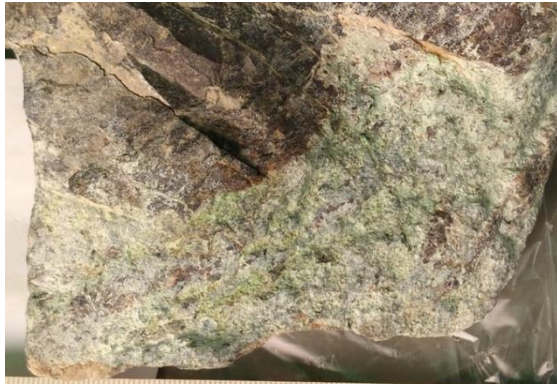
Stringers of Co-Ni mineralization in low grade metamorphic sediments
