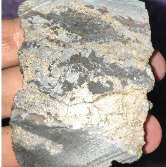
Stringers of Co-Ni mineralization in low grade metamorphic sediments
